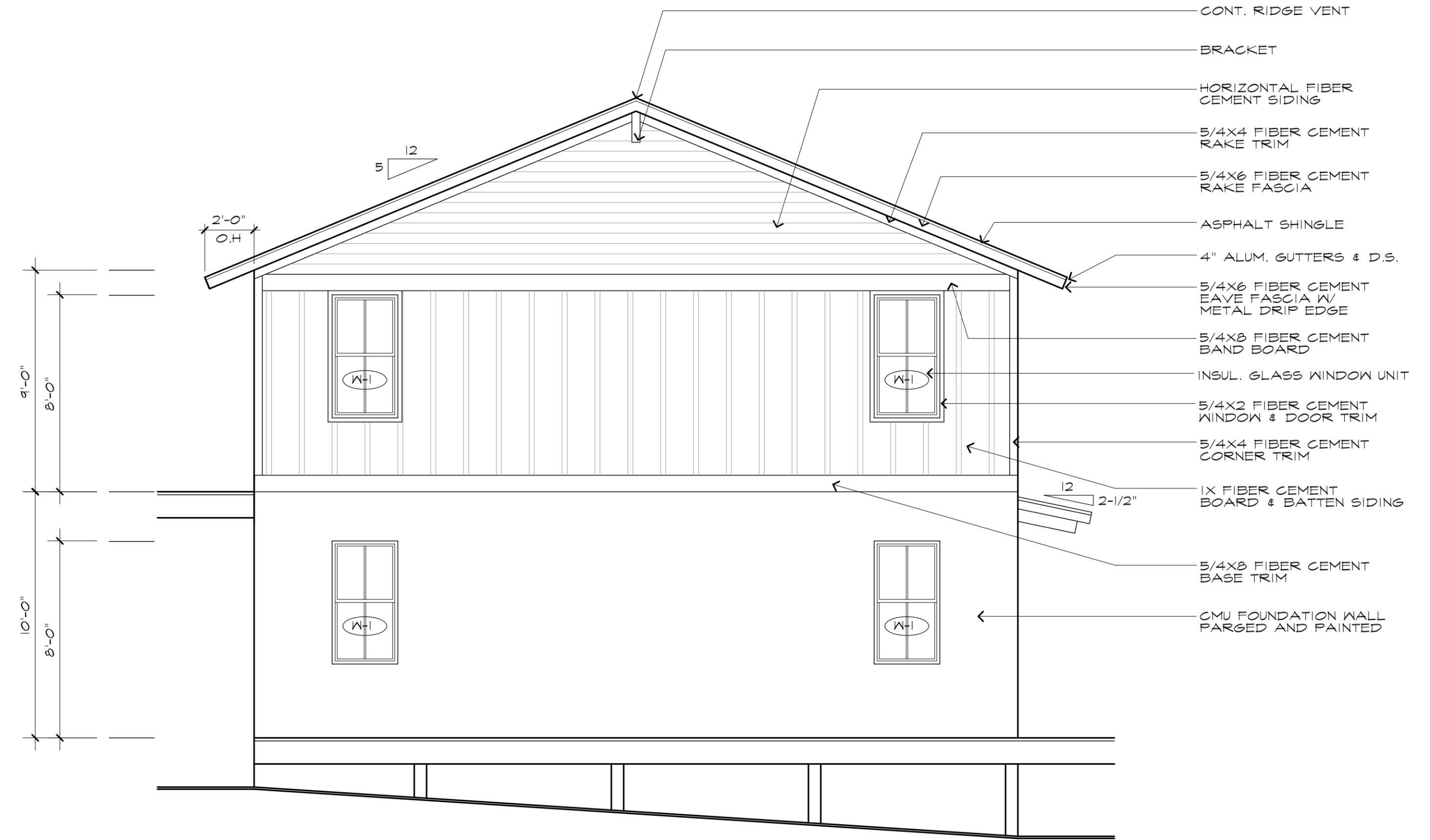
2 BUILDING D3 - RIGHT ELEVATION
